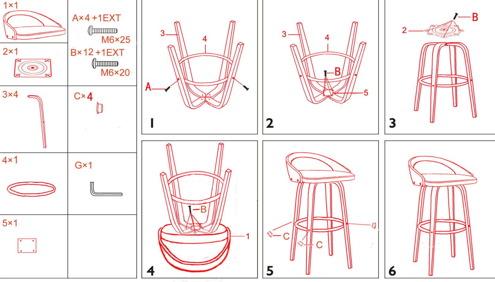
Noted: 1.Lightly tighten the screws indicate on step 1&step 2 &step 3.
